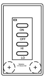
Two #2032 Button Batteries power the wall control transmitter They are available at your local hardware store.
