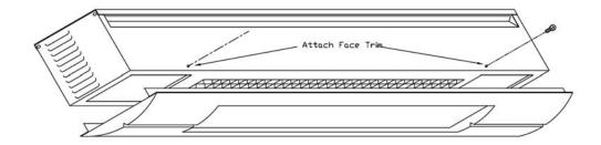
Optional Face Trim can be easily installed on all Sunpak models.
