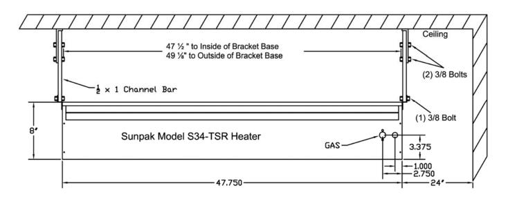
Warning: Heater must be level in the lengthwise direction.
