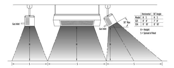
SUNPAK will raise the comfort level 5-10° Fahrenheit outdoors. The above coverage table was based on still breeze conditions. Under windy conditions more heat will be required. It is recommended that a windswept patio be designed with wind breaks to stabilize the patio environment. Wind breaks shall NOT interfere with the ventilation or combustion air requirements of the heater(s) and meet clearance for combustible requirements listing on page 6 & 7.
