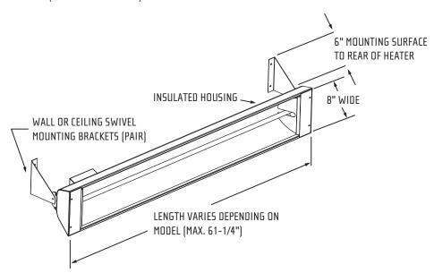
Wall/ceiling brackets are furnished with all heaters. Their use is optional. When used, they allow heater to be fastened to wall or ceiling and then tipped up to 60°. Heater can also be hung in a horizontal position using chains or custom brackets. Heater must be level, but can be rotated around its horizontal axle.
