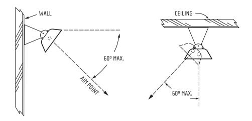
NOTE: DO NOT mount the heater on a vertical axis. Such installation will reduce the life of the element and will automatically void the product's warranty. Heater must be installed with the quartz tube horizontally level. For maximum tube life, use a carpenter's level tool to find the optimum level position for the heater's body. Always maintain the minimum clearances from the heater body to any combustible materials.
