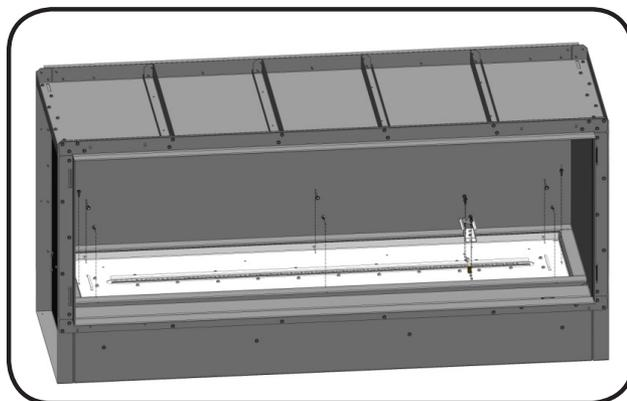
Remove the flex hose and the orifice from the burner and completely remove the glass tray from the fireplace.
