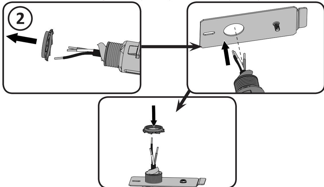
Connect the ground green wire to the junction plate using the grounding screw (W570-0098). Using the wire connectors, connect the common white wires together, then the hot black wires.
