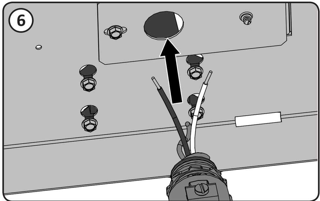
Connect the Green ground wire to the junction plate using the ground screw as shown. Connect the common white wires together as shown, followed by the hot black wires as shown.
