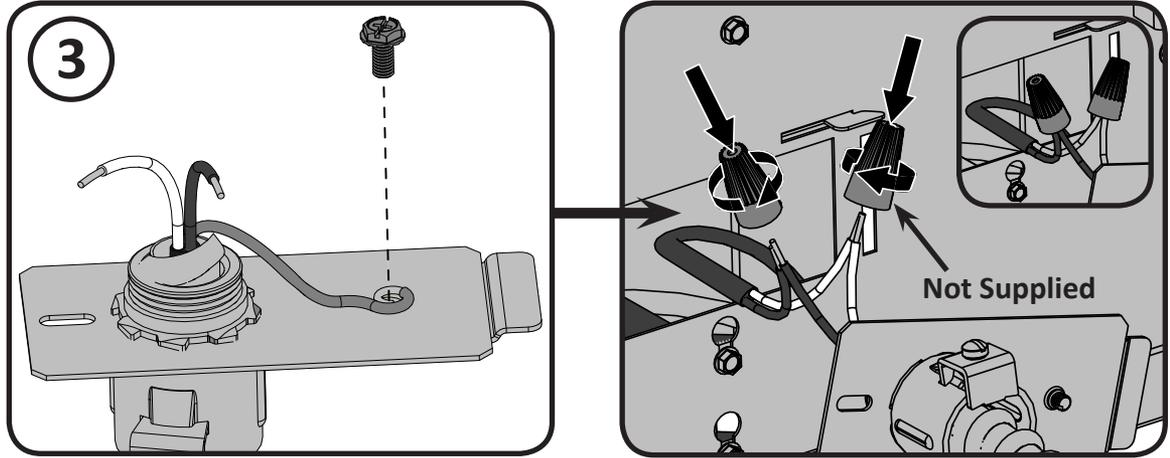
Reinstall the cover plate using the screw (N570-0008), as shown.
