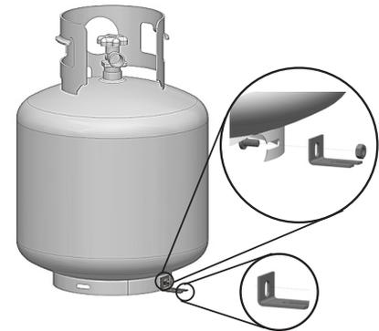
**Cylinder Connection:** Ensure the gas regulator hose is kink free. Remove the cap or plug from the cylinder fuel valve. Insert the black QCC1 regulator nipple onto the QCC1 fuel valve. Hand tighten clockwise. Do not use tools. Leak test all joints prior to using the appliance. A leak test must be performed annually and each time a cylinder is hooked up or if a part of the gas system is replaced.
