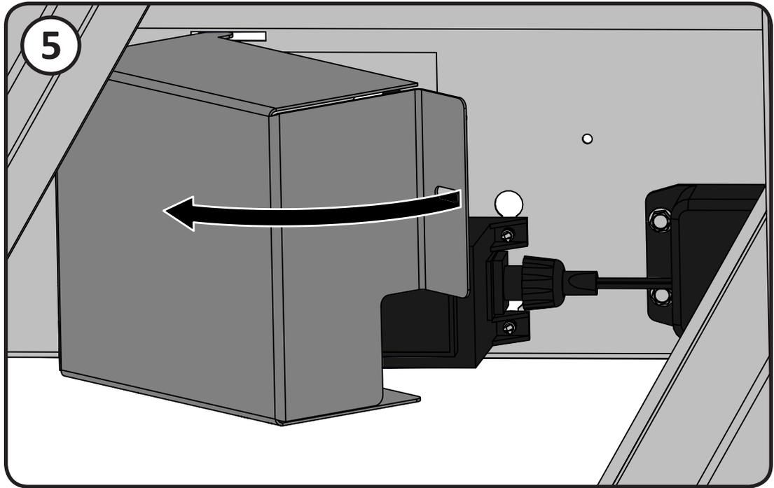
Install the box connection using the 7/8" (22.2mm) hole in the junction box.
