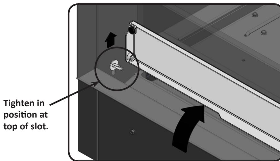
4. Line up the brackets on the trim with the slots on the side of the base and insert as illustrated pushing until trim sits flush against front surface. The brackets have been designed with multiple slots (1/4" (6mm) increments) to accommodate different finishing materials.
