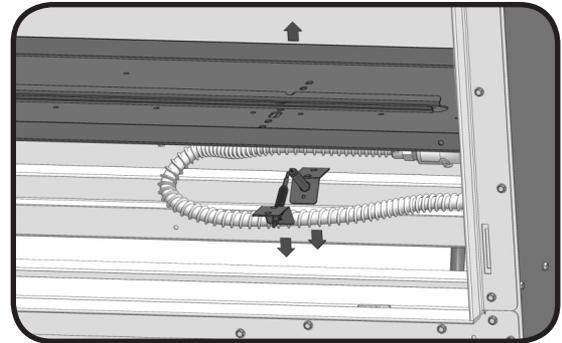
4. Disconnect the stainless steel flex connector from the orifice using (2) wrenches.
