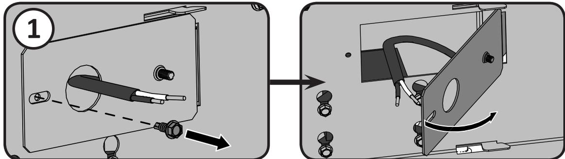
Install the box connector through the 7/8" (22.2mm) hole and into the junction plate.
