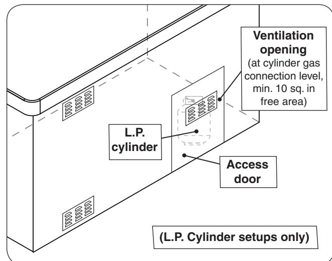
Fig. 9-2 Additional ventilation opening for L.P. cylinder
