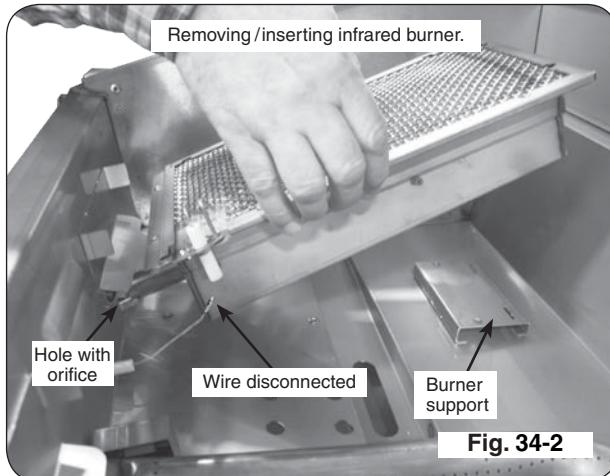
4. Use a  $\frac{1}{2}$ " hex nut driver to remove the exposed orifice. Access it through the hole in the forward firebox plate inside the grill (Fig. 34-2). Check orifice. If needed, replace it with the correct orifice for the new gas.
