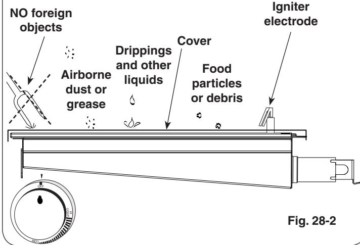
Burner ceramic must be protected with cover when burner is not in use.
