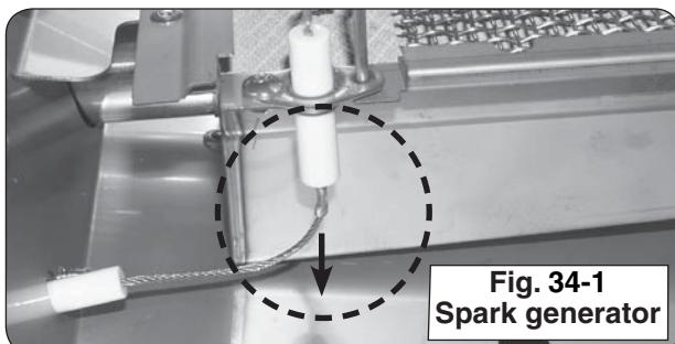
6. Reconnect the ignitor wire to the bottom of the electrode assembly on the infrared burner.
