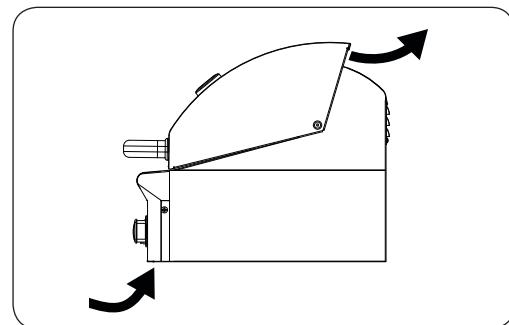
Fig. 12-1 Airflow diagram
