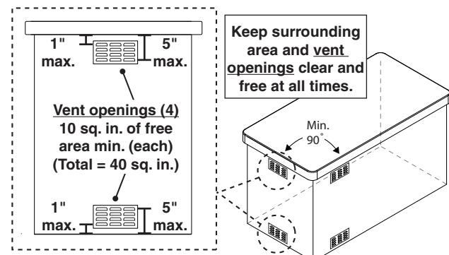
Fig. 8-1 Ventilation detail
