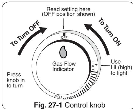
**Note:** **DO NOT** turn on more than one valve at a time for either electronic or manual lighting.
