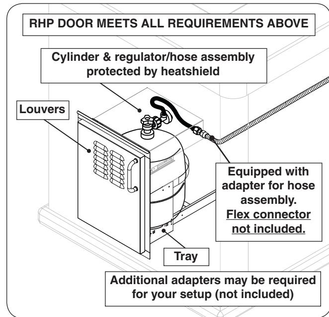
Fig. 9-3 Optional AOG door w/ tank tray & louvers
