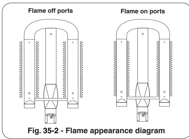
Fig. 35-2 - Flame appearance diagram
