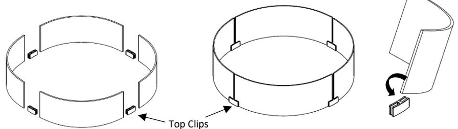
**NOTE: Glass Guard should be assembled upside down, and flipped over after assembly.**
